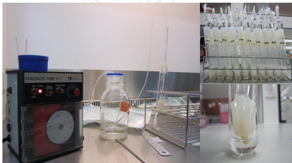
Figure 6 Preparation of glucose filtration test
