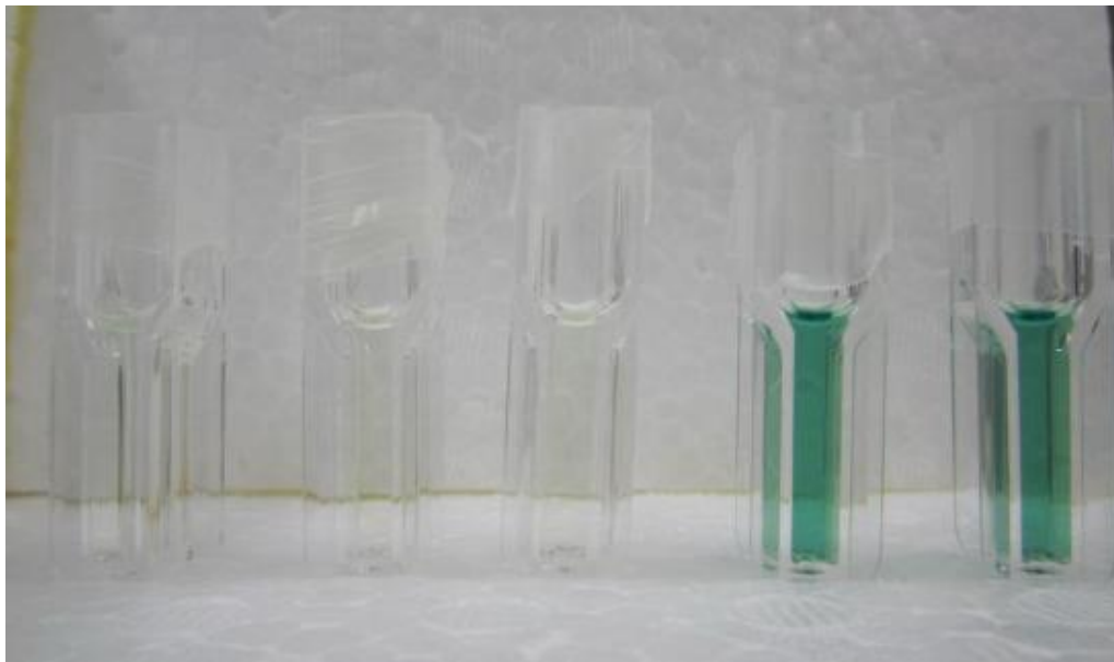
Figure 10 The three cuvettes on the left demonstrated detected color of the negative control and the two cuvettes on the right demonstrated detected color of positive control in glucose infiltration test
