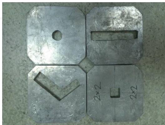
Figure 3. 5. The various shape and size of cutout shields insert in a 10 \times 10 \text{ cm}^2 standard cone.
