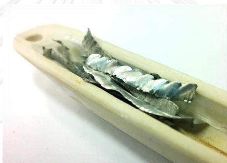
Figure3.2 zinc dross supplied by FOSECO (Thailand)
