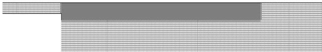
Figure3.7 Grid generation in 2-D simulation domain
