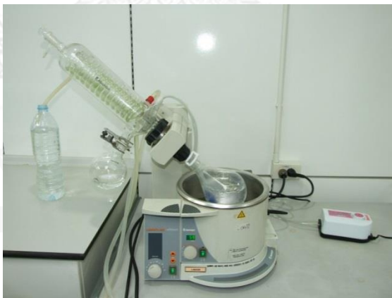
Figure 21 Experiment setup for \text{NH}_4\text{HCO}_3 removal
