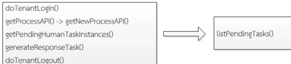
Figure 5.2 The caller listPendingTasks do not re-write code when operations have been changed
