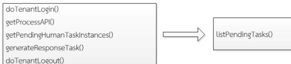
Figure 4.6 Five method are encapsulated into listPendingTask
