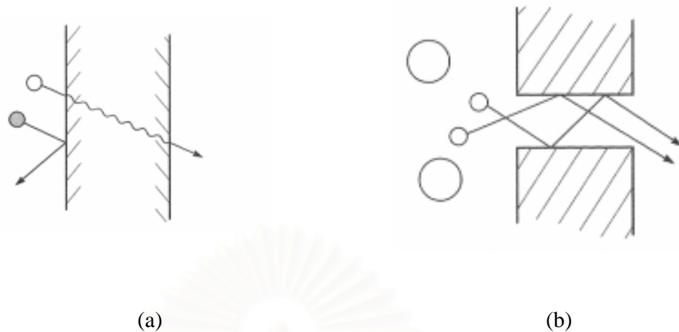
Figure 2.3 Schematic of molecular transport through membrane: (a) molecular diffusion and (b) molecular filtration (Baker, 2004; Suntarapha, 2004)
