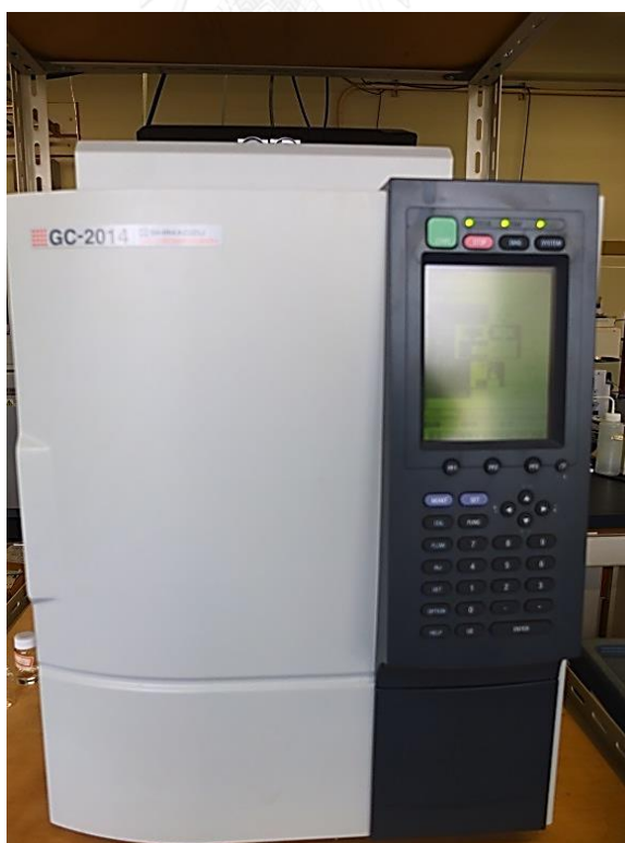
Figure 3.10 Gas chromatography-Flame ionization detector (GC-FID) with a silicone SE-30 column for liquid products analysis
