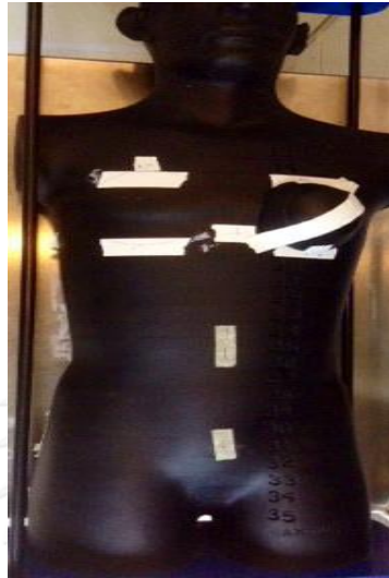
Figure 3.7 Alderson Rando phantom
