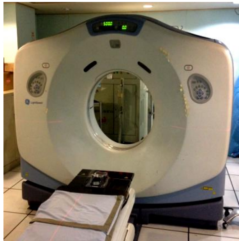
Figure 3.3 CT simulator scanner with 4 slices (GE LightSpeed RT)
