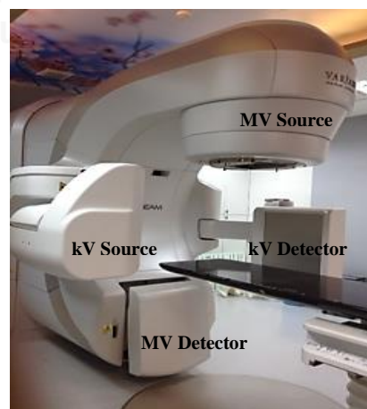
Figure 3.4 Varian TrueBeam linear accelerator with the OBI system
