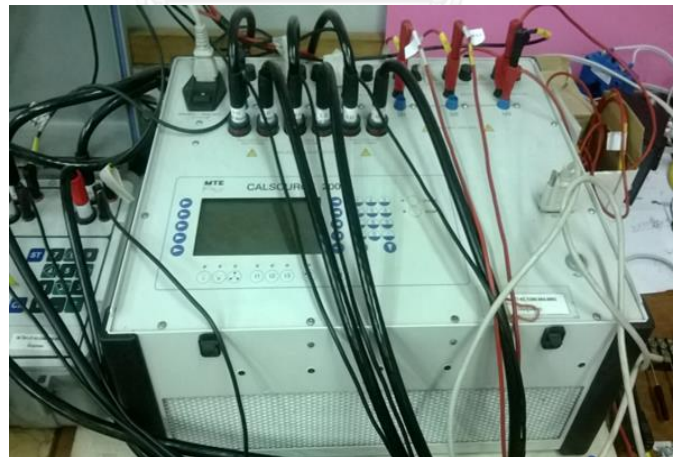
Figure 5-1: MTE-CALSOURCE-200, programmable 3phase power supply
