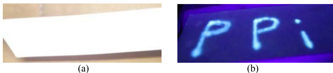
Figure 4.29 Image patterns of L2•Zn dipped with PPI solution on a filter paper (a) in the visible light and (b) under UV irradiation at 365 nm.
