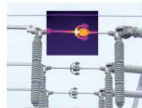
Fusion, a function that lets you display a part of digital photo as an infrared image.
