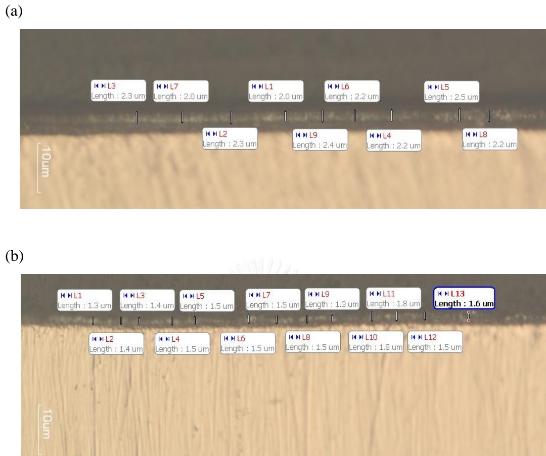
Fig. 4.15 Thickness measurement by optical microscope of the selective specimen; (a) as-deposited and (b) 300°C annealed CoFe film with 80.0 wt.% Fe.
