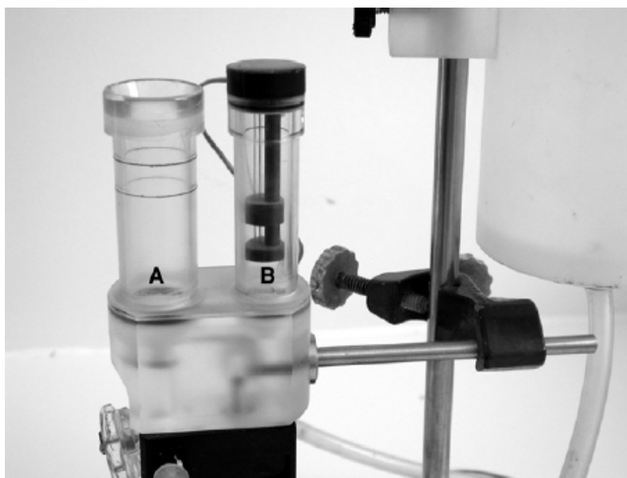
Figure 17 Plethysmometer. The larger one (A) is used to measure fluid displaced by the paw, a volume change that is precisely mirrored in the smaller tube (B) containing a transducer which is linked to a decoder capable of digitally displaying volumes.
