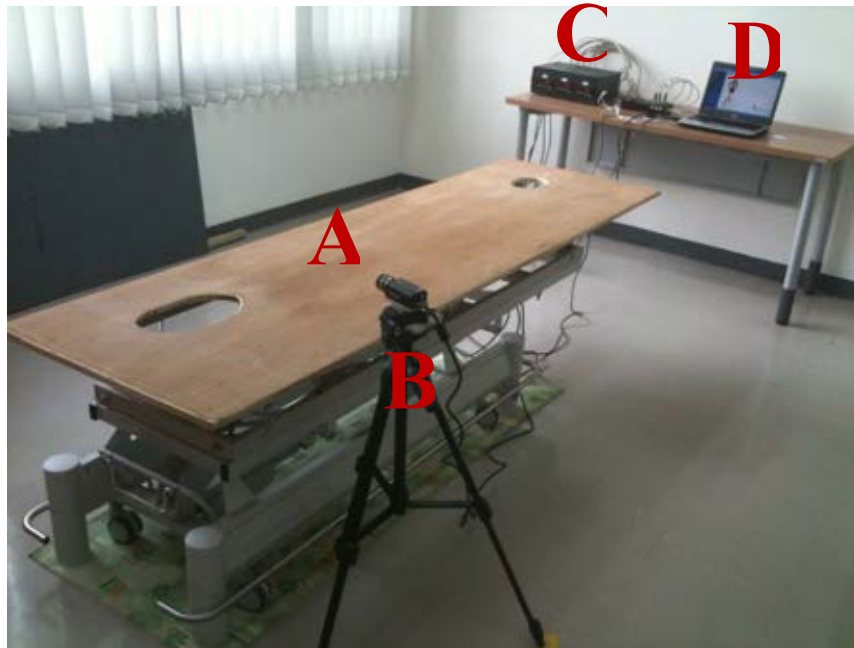
Figure 3.1 The instrumentation of the study. A, B, C and D represent a custom made couch, a motion capture system, a display box and a computer, respectively.
