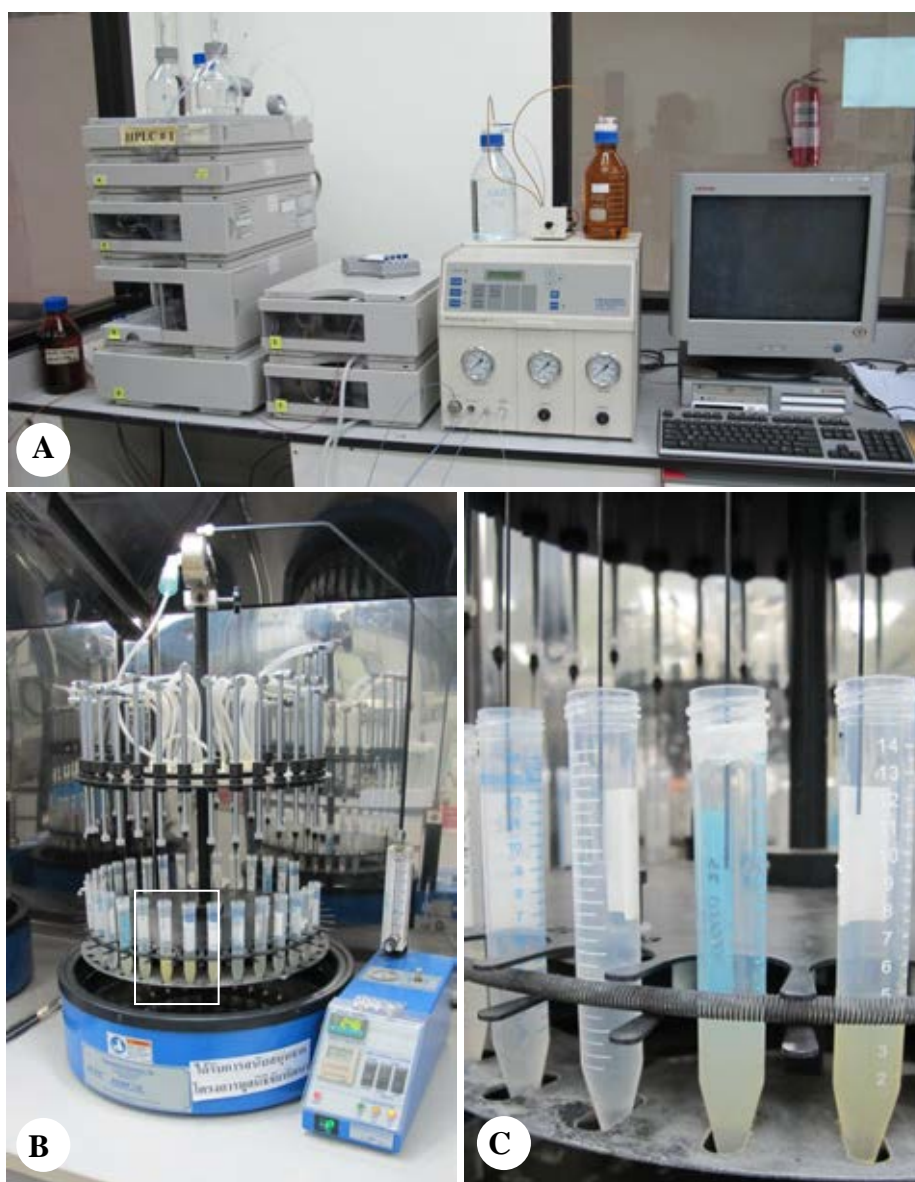
Figure 3.2 A High Performance Liquid Chromatography (HPLC), B-C Evaporator
