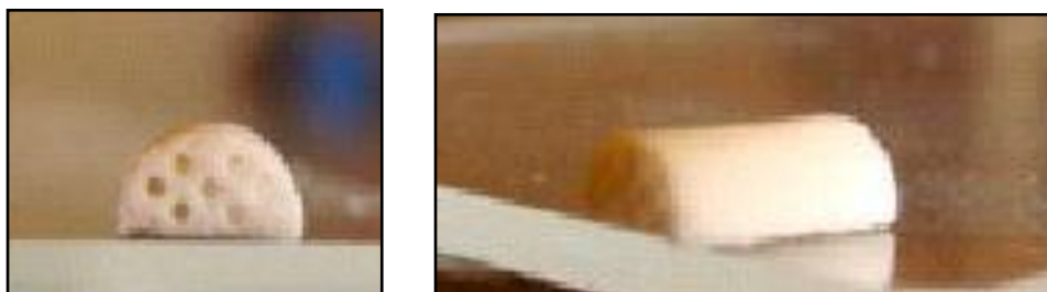
Figure 2.5 250 \mu\text{m} multichannel bridges are fabricated using a gas foaming process microspheres (PLGA) [43].
