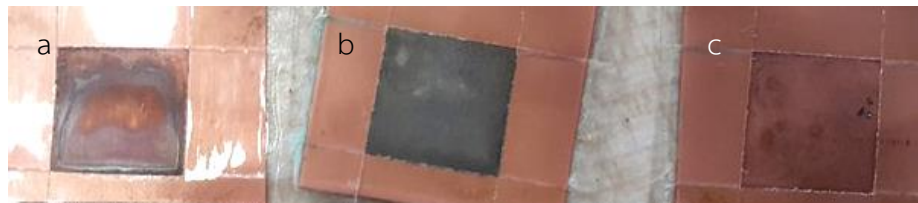
Figure 6.2 The uneven plating (a, b) and skip plating (c) defect from iron contamination
