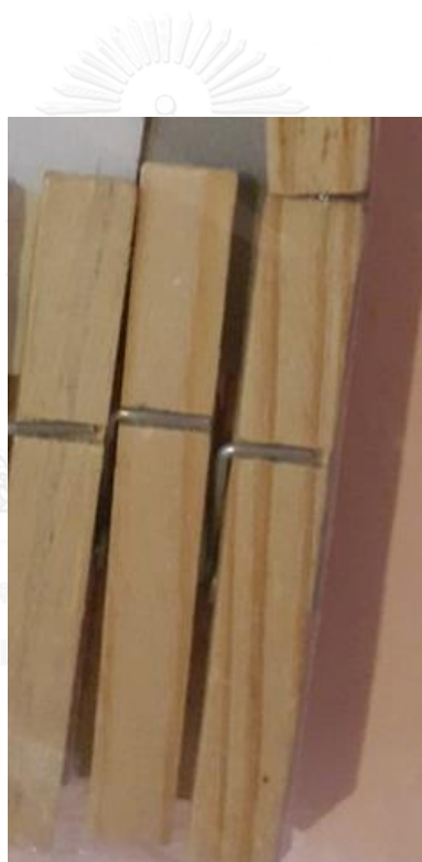
Figure 6.1 The wood peg which was used to grip the substrate
