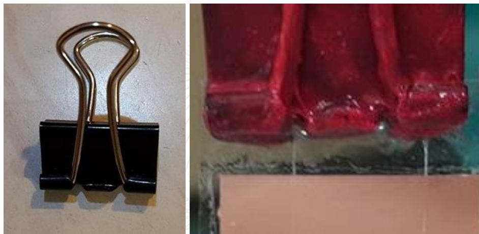
Figure 6.3 The double clip (left) and double clip coated by nail polish (right)
