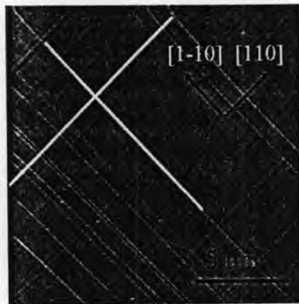
Figure 4.1 AFM image of the surface of In 0.15 Ga 0.85 As layer on GaAs (001) substrate.
