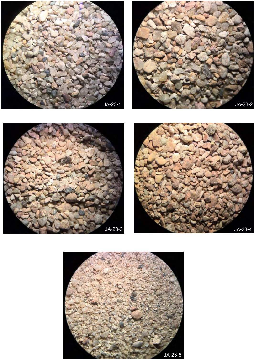
Figure 4-19 Photo of cutting samples from the well JA-23 (4X magnification).
