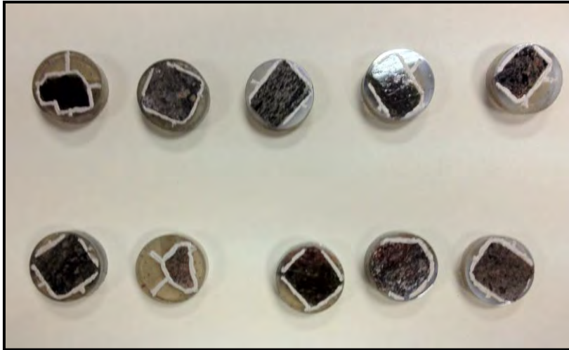
Figure 2.14 Selected polished epoxy plugs for EPMA analysis
