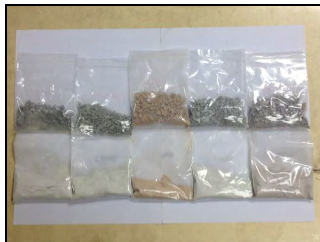
Figure 2.13 Rock powdered samples for XRF and XRD
