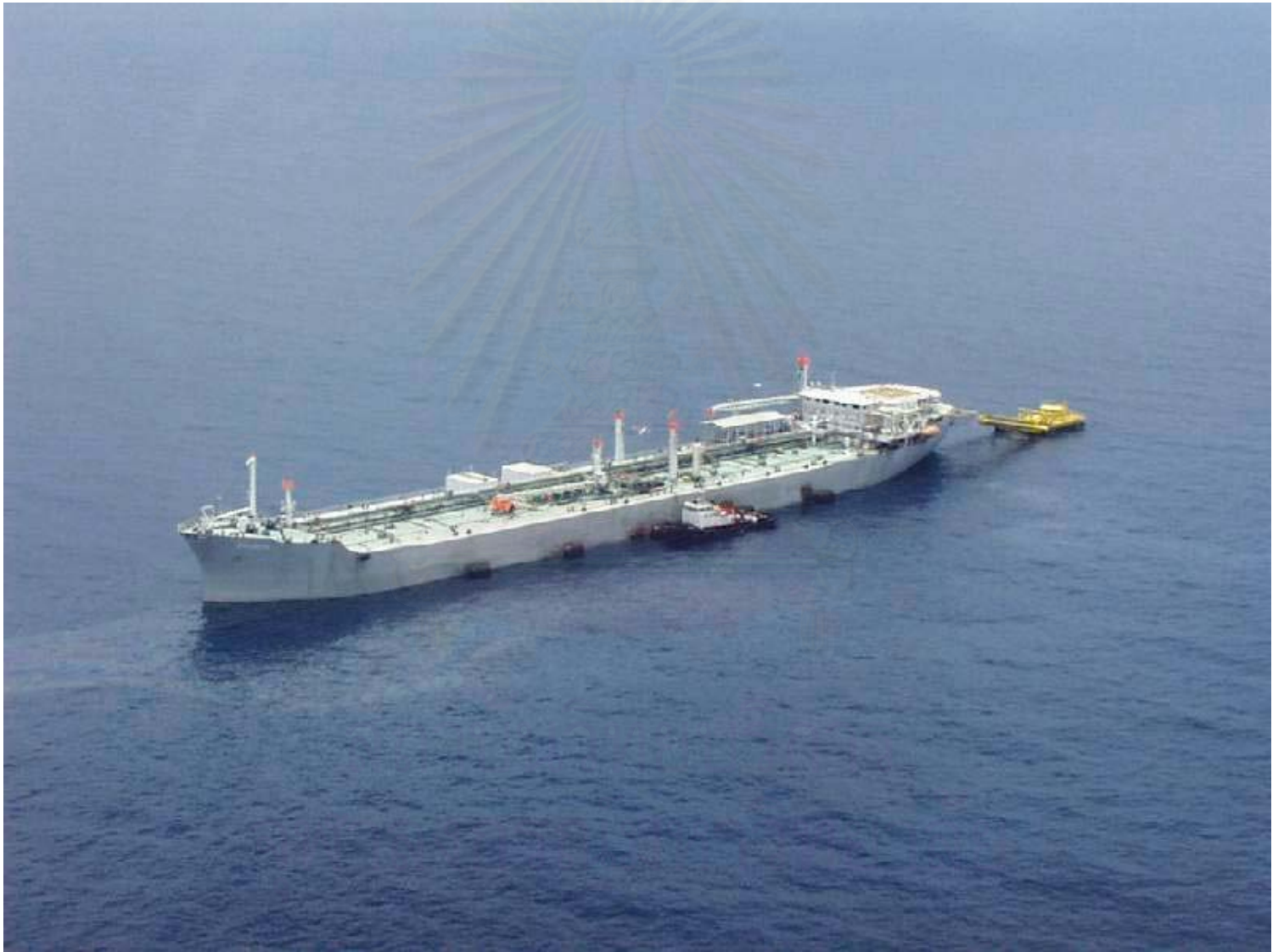
Figure 4.1 : FSO - Floating Storage and Offloading
