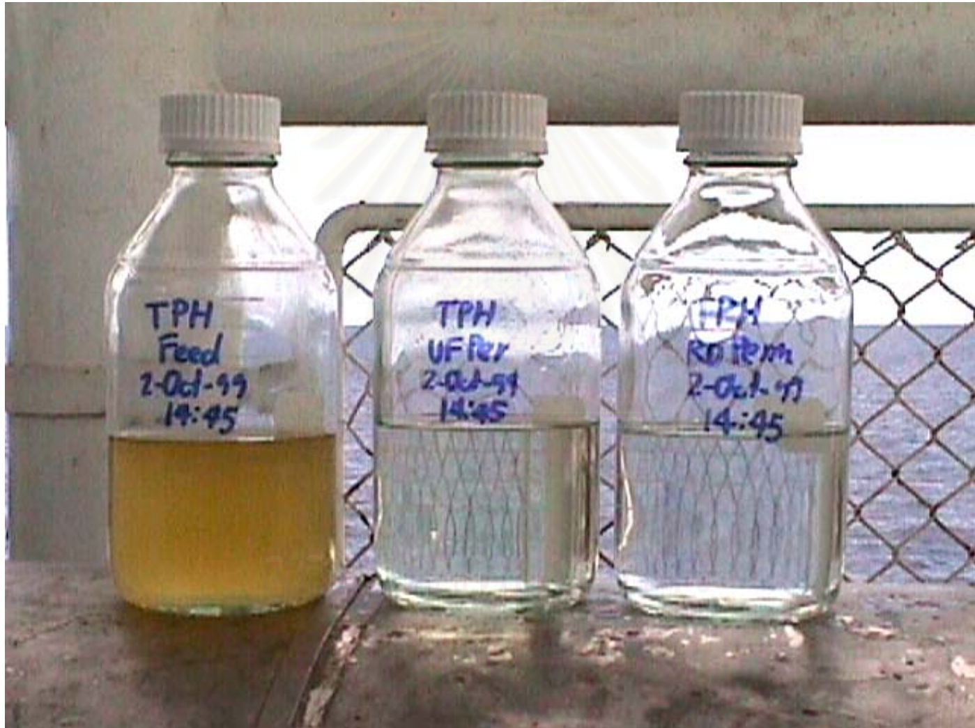
Figure 5.1 : Photo of Membrane Pilot Plant Feed and Product Water
