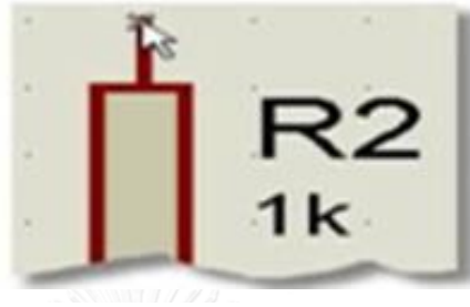
Figure B 8. The Mouse cursor indicating that the mouse is over the pin tip
