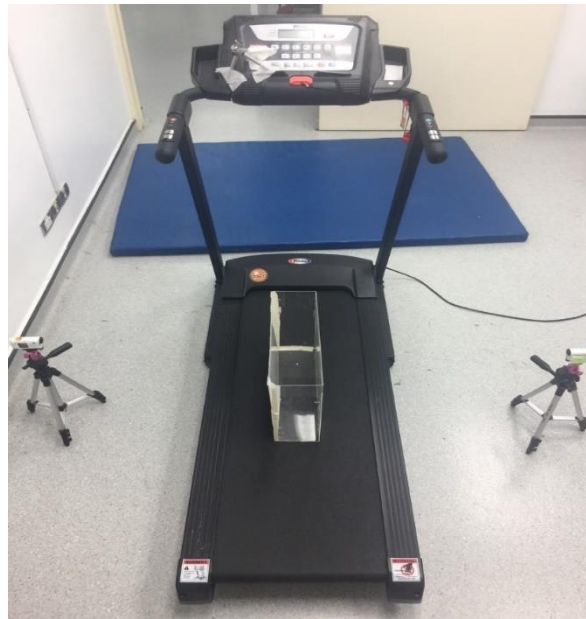
Figure 5 Kinematic system and cameras position for recording the kinematic data on top view
