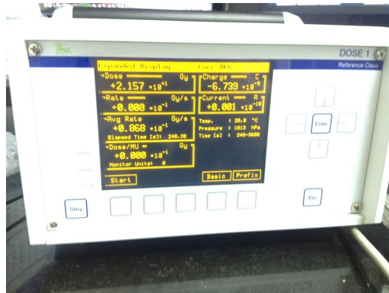
Figure 3.21 The Dose-1 electrometer with +300 volt.
