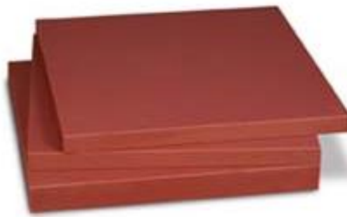
Figure 3.4 The virtual water slab phantom.
