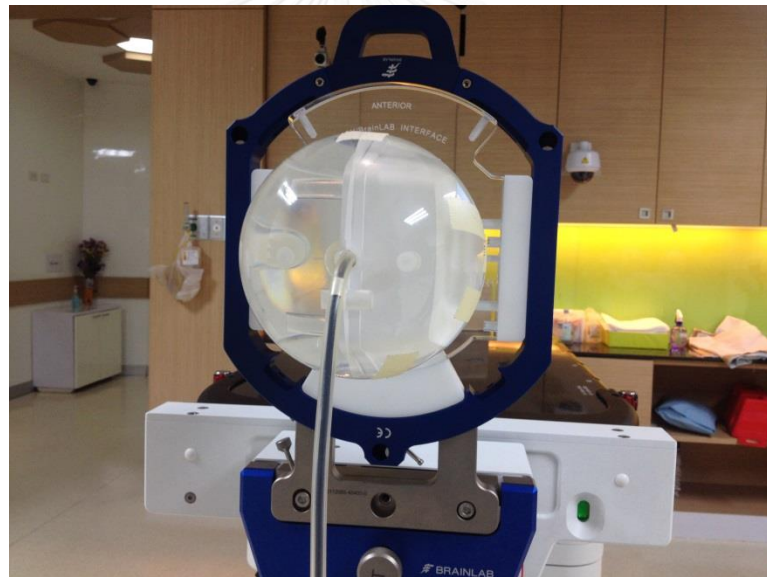
Figure 3.20 The CC01 ion chamber inserted in Lucy phantom.
