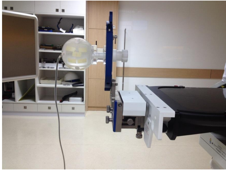
Figure 3.19 The CC13 ion chamber inserted in Lucy phantom.
