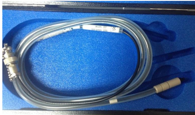
Figure 2.10 The ionization chamber (IBA CC01 ion chamber).
