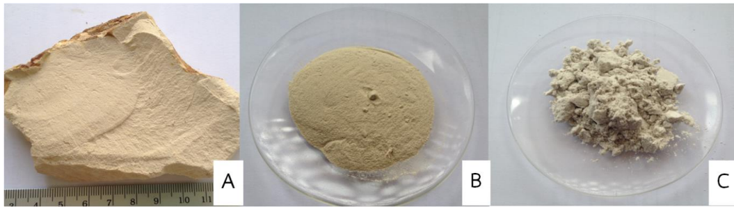
Figure 3.1 : Geomaterials used to make the adsorbents. (A) siltstone, (B) soil sample, and (C) expanded perlite.
