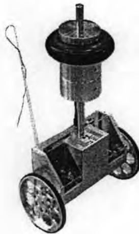
Figure 1.1: JOE: mobile inverted pendulum.
