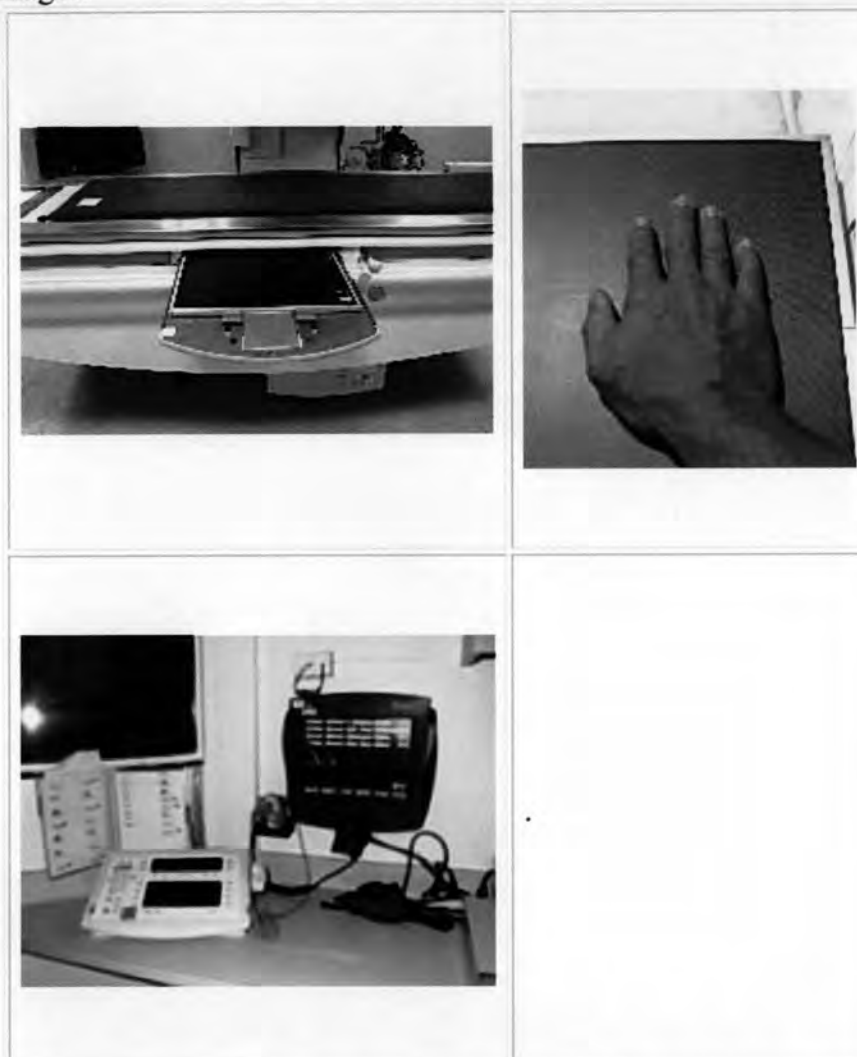
Figure 12. CR cassettes. Above, the same cassettes can be used in the bucky tray or tabletop. Left, by placing ROP's in locations near the exposure console, the technologist is able to enter and approve images between radiographic exposures
