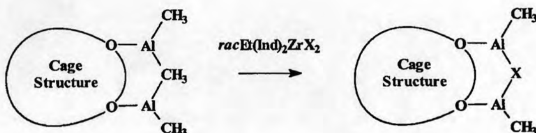
Figure 2.13 Representation of MAO showing the substitution of one bridging methyl group by X ligand extracted from \text{racEt(Ind)}_2\text{ZrCl}_2 (X = Cl, NMe 2 , CH 2 Ph) [19].
