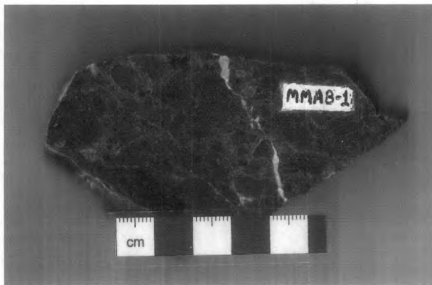
Figure 4.5. Slab of monomictic andesitic breccia (sample no.MMAB-1) showing only one type of dark-colored volcanic fragment at the Chatree gold min, Phichit. Note that the breccia rock was cross cut by calcite vein.
