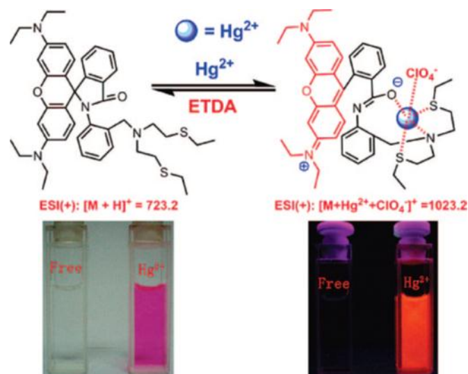
Figure 1.10 Proposed binding mode between sensor/ \text{Hg}^{2+} and color change upon addition \text{Hg}^{2+} .
