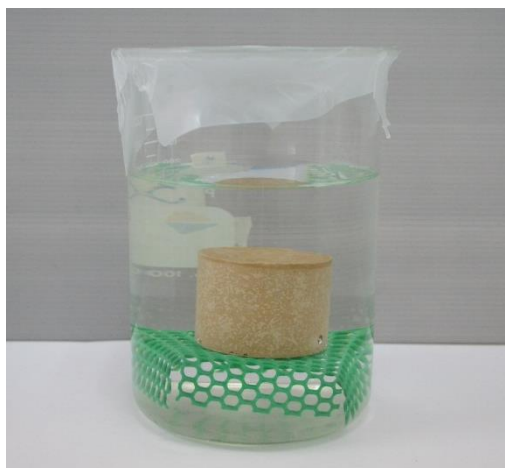
Figure 4.23 Photograph of test portion in leaching process.
