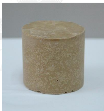
Figure 4.22 Solidified waste sample (6:4 of cement to contaminated sludge ratio).
