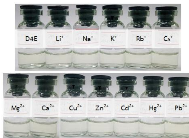
Figure 3.11 Color of 1 \times 10^{-4} M D4E upon addition of 10 eq of metal ions
