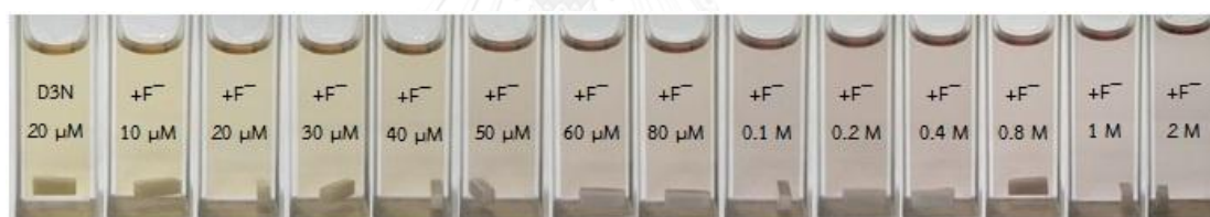
Figure 3.24 Color of 20 \mu\text{M} D3N upon the addition of various amount of \text{F}^- in DMSO
