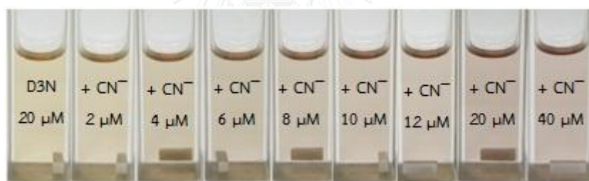
Figure 3.26 Color of 20 μM D3N upon the addition of various amount of CN - in DMSO
