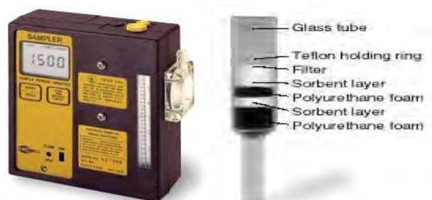
**Figure 3.1** Personal Pump and sorbent (OVS-2) tube
