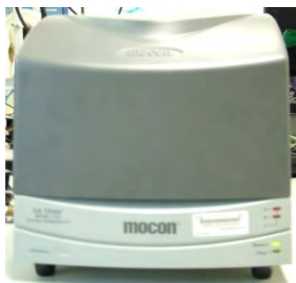
Figure 4.1: Oxygen permeation analyzer; OX-TRAN 2/21, Mocon, USA
