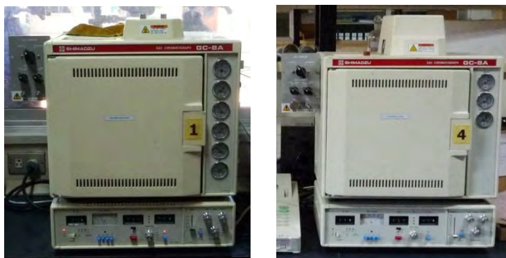
Figure 4.4: Gas chromatograph for C_2H_4 (a) and O_2/CO_2 (b) test; GC-8A, Shimadzu, Japan
