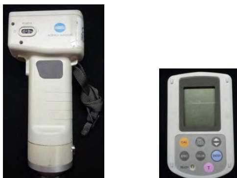
Figure 4.5: Color meter; Minolta CR-400, Konica Minolta Sensing, Japan
