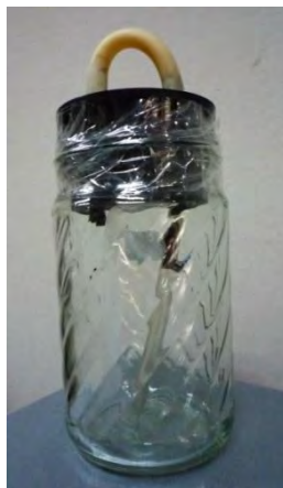
Figure 4.3: The equipment of ethylene adsorption test
