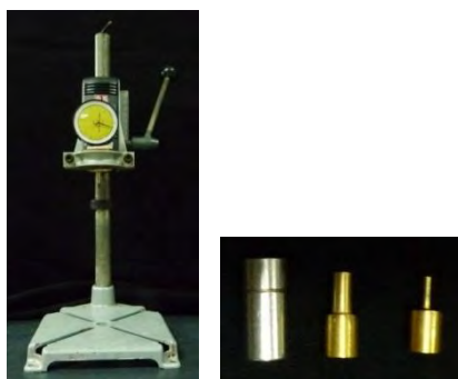
Figure 4.6: Fruit firmness tester; Black&Decker, and probe with various sizes
