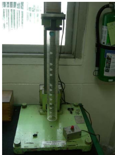
Figure 4.3 Auto Urethane H/N Tester
