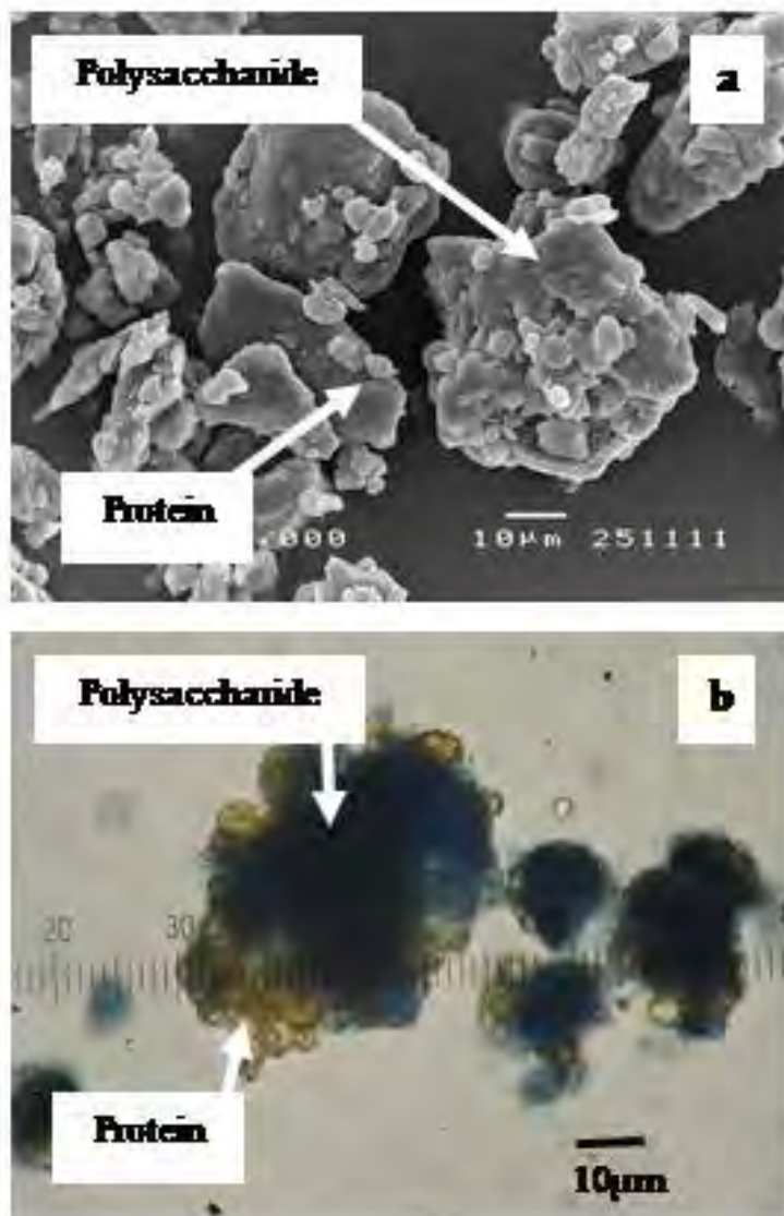
Figure 5.1 (a) Scanning electron microscope images of tamarind kernel powder, (b) Microscope images of tamarind kernel powder dispersed in water.
