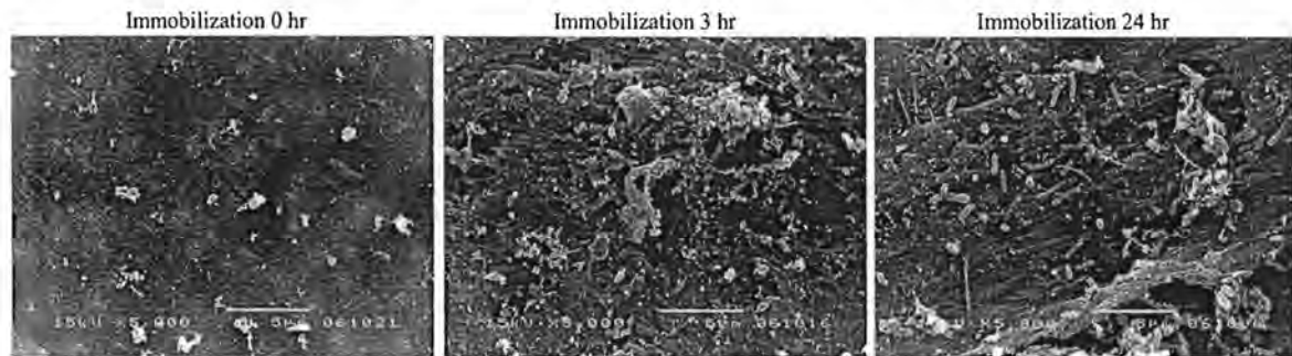
Fig. 4 SEM images of bacteria immobilizing on chitosan after immobilization for 0, 3 and 24 hr.
