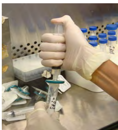
C. Filtrating the micelle fraction
