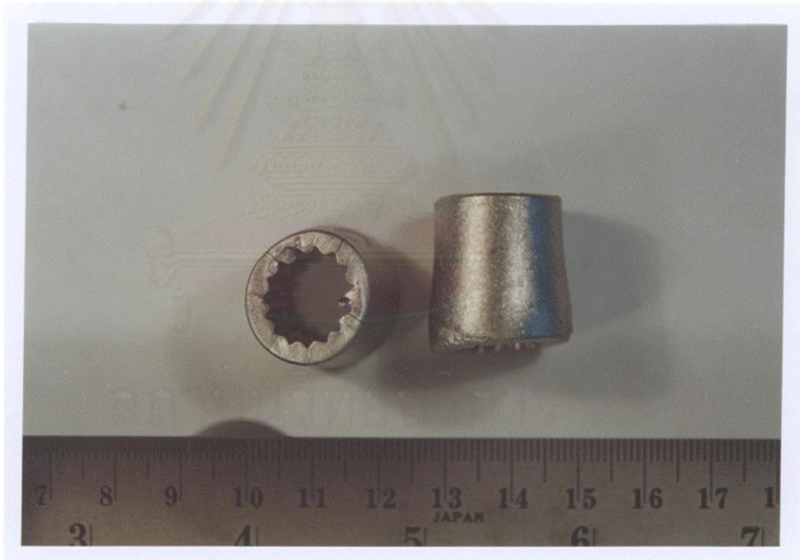
Figure 4.7 Photograph of splined coupling which debound in condition 10
