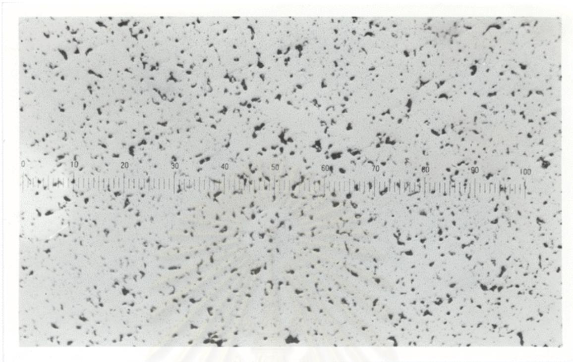
Figure 4.5 Pore structure of a tensile specimen which sintered at 1195°C in  $N_2+70\%H_2$  atmosphere (x200)
