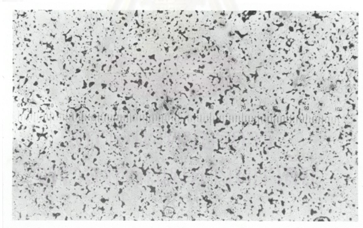
Figure 4.6 Microstructure of a tensile specimen which sintered at 1195°C in  $N_2+70\%H_2$  atmosphere (x200)
