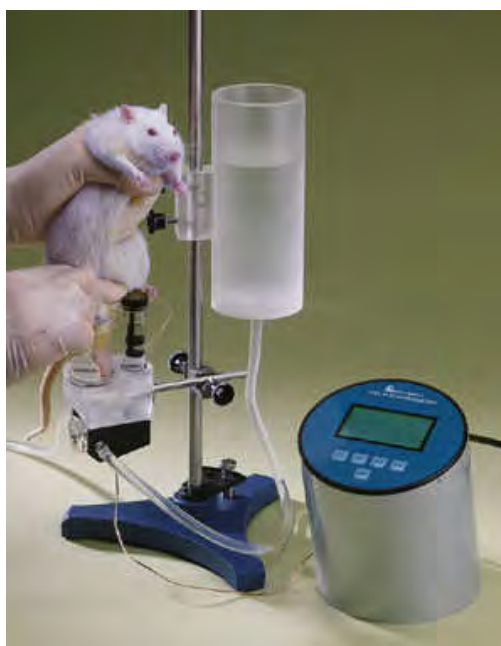
Figure 9 Plethysmometer, an apparatus for the measurement of rat paw volume
