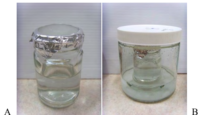
Figure 11. WVTR bottle containing water and covered with hydrogel membrane (A), The humidity controlled chamber for the WVTR bottle (B)
