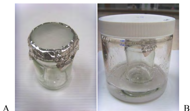
Figure 12. WER bottle covered with hydrogel (A), The humidity controlled chamber for the WER bottle (B)
