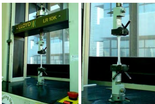
Figure 37. Mechanical properties of the PVA and DG/PVA hydrogels tested by LLOYD instrument
