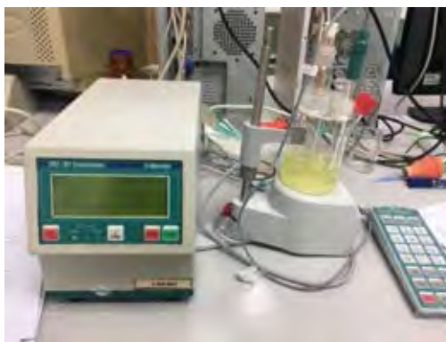
Figure 3.6 Water content measurement by Coulometer 831 KF.
