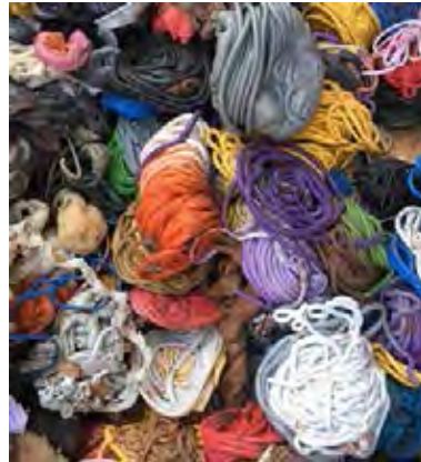
Figure 4.8 Industrial cable wastes from extrusion process.
