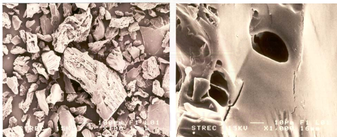
Figure 4.28 SEM micrograph of poly(acrylic acid- co -acrylamide) synthesized with formaldehyde crosslinking agents (Water absorbency = 238 \pm 12 \text{ g g}^{-1} )
