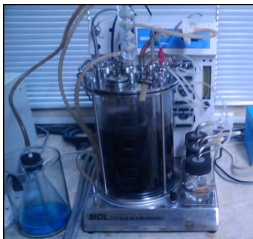
Fig. 3.3 Ethanol production in 5 liter fermenter
