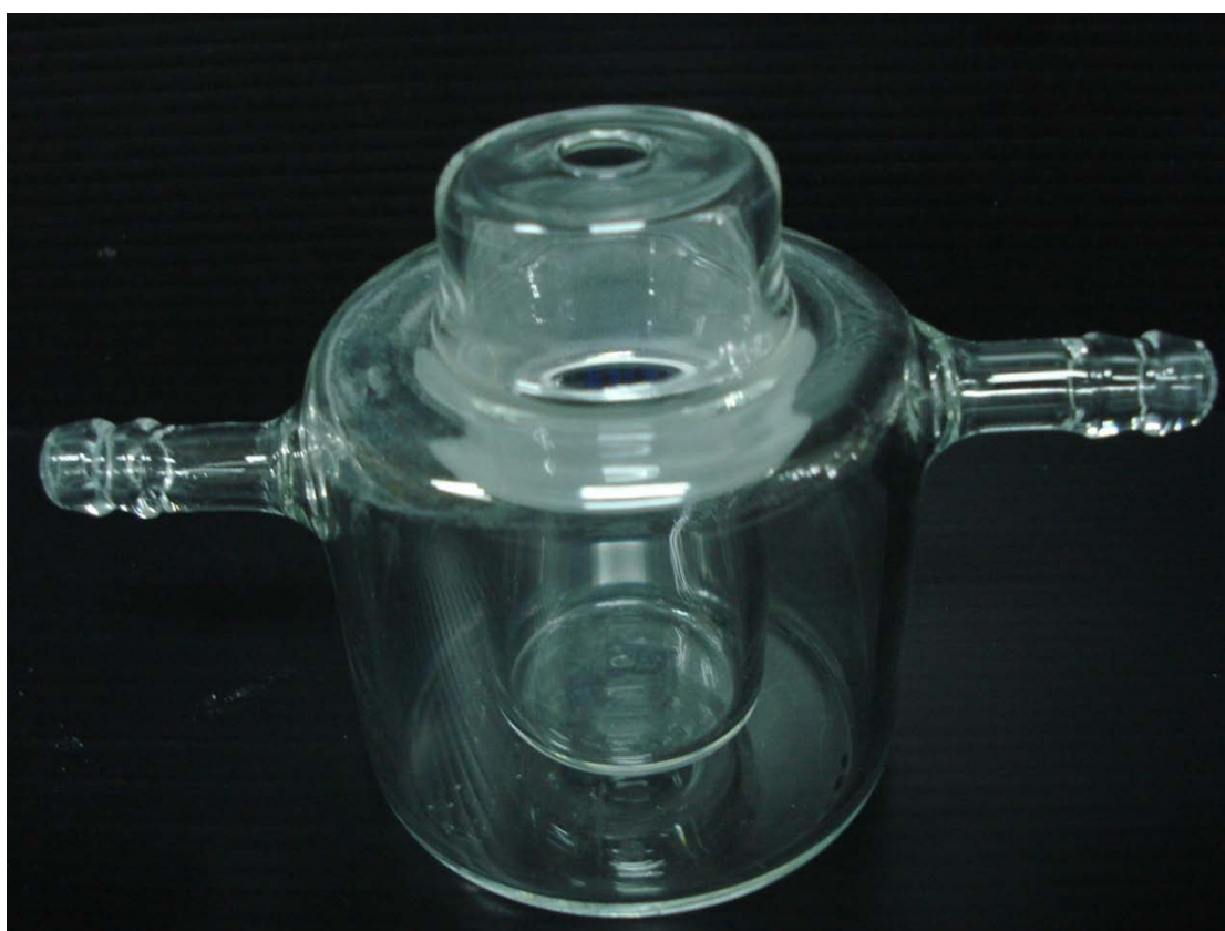
Figure A1: A closed water-jacketed glass cell for preparation of ethosomes
