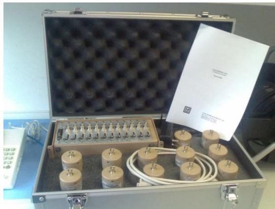
Figure 3.1 Radiation counter system with 12 NaI detectors.
