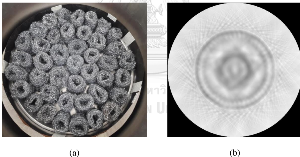
Figure 4.23 (a) Arrangement of simulated packed bed structure without scale deposited and (b) reconstructed image of structure without scale case.
