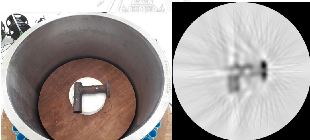
Figure 4.31 Experiment phantom broken pipe with flange
