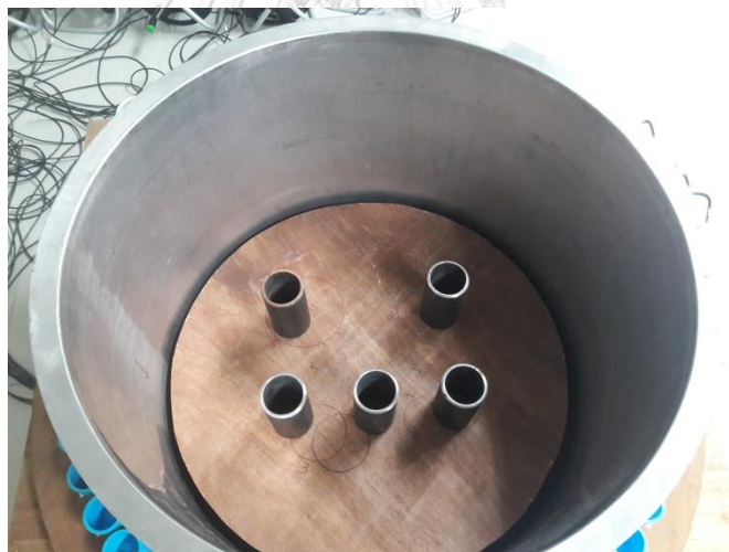
Figure 4.29 Experiment phantom broken pipe with flange
