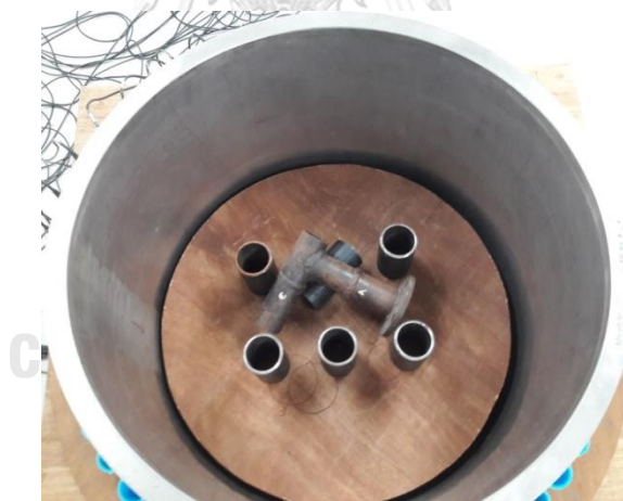
Figure 4.32 Experiment phantom broken pipe dropped down and damage six riser pipes
