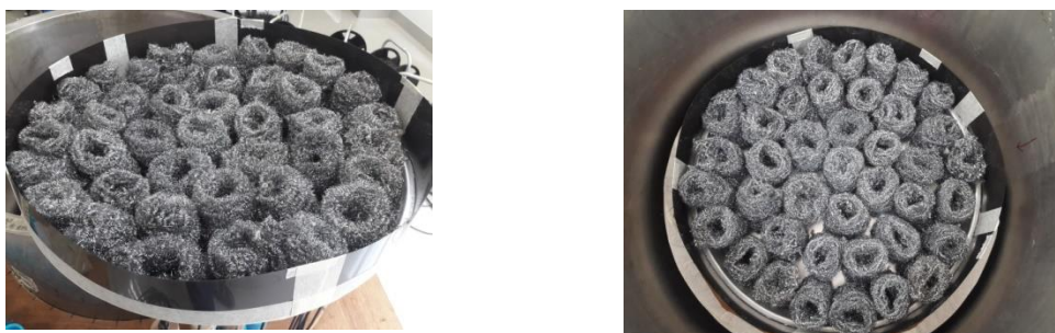
Figure 4.22 Arrangement of simulated packed bed structure
