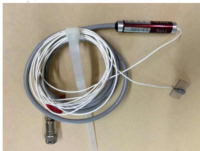
Fig. 4-12 PWP sensor and accelerometer
