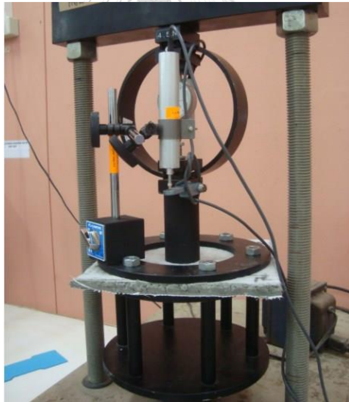
Fig. 3-10 Puncture test setup
