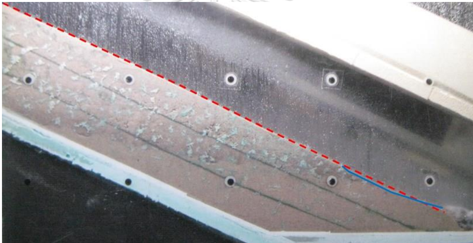
(c) Case 3: Unreinforced slope under rainfall, t = 3.0 min
