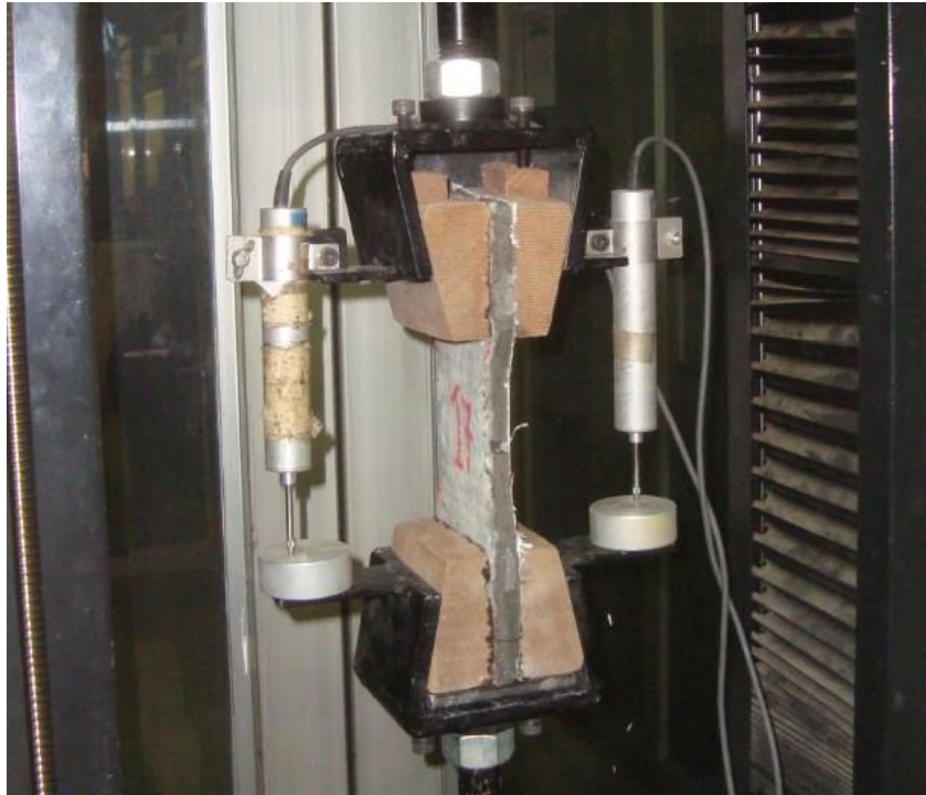
Fig. 3-6 Geometry of specimen and tensile test set up
