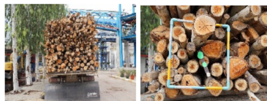
Fig 1. An example image of a timber truck and reference diameter template on log end.
