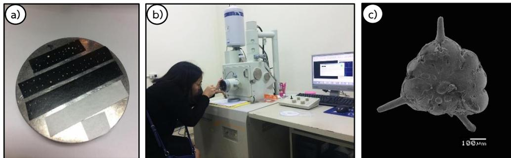
**Figure 3.17** The study of fossil identification by scanning electron microscope (SEM) following a) Microfossils that were sort out under microscope for study by scanning electron microscope (SEM) were arrayed on the stub before put into the scanning electron microscope (SEM), b) Putting the stub that cover with microfossils into scanning electron microscope (SEM), and c) The picture of microfossil by scanning electron microscope (SEM) was prepared for species identification.
