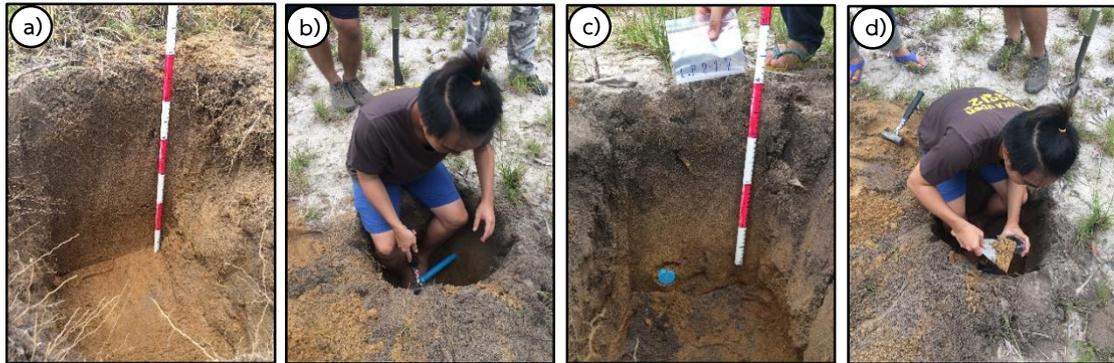
**Figure 3.7** The steps of sediment sampling for OSL dating in laboratory which consist of a) Digging an excavation pit at 50x50x50 cubic centimeters, b) Putting pvc tube with end cap at depth 40 centimeters from surface, c) Pvc tube with end cap was put into sediments layer at depth 40 centimeters from surface for sampling sediments for equivalent dose evaluation, and d) Sediments were sampling at depth 40 cm in plastic bag for annual dose calculation.
