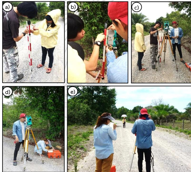
**Figure 3.6** The topographic profile was measured by Total Station SOKKIA SET 630R along transect lines. These pictures consist of a), b), c) The measurement of pole, total station, and tripod respectively before start the topographic survey for calculation with elevation further, d) and e). The topographic profile measurement was done by Instrument man, staff man (rod man), and recorder.
