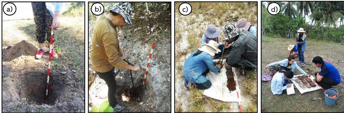
**Figure 3.8** The steps of stratigraphic column for analyzing sediment deposition and paleo-environment which consist of a) Digging an excavation pit at 50x50x50 cubic centimeters, b) Sampling sediments with hand auger, c) After sampling sediments with hand auger, put sediments in the on the plastic sheet for logging description, and d) Description of sediments which include of depth, color, composition, and other evidences.
