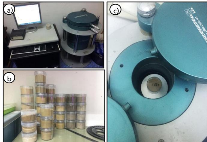
**Figure 3.19** The steps for annual dose calculation by gamma ray spectrometer following a) Gamma ray spectrometer, b) Sediment samples in plastic boxes are prepared for putting in gamma ray spectrometer, and c) Putting the box into gamma ray spectrometer and start calculation.
