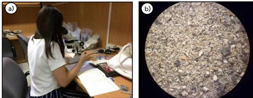
Figure 3.12 Sediment compositions analysis in laboratory room. a) Using a binocular microscope for classifying sediment compositions. b) Sediments sample under the microscope.
